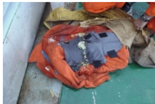
Photo 04 – After UHP jetting , the PVC cloth, was destroyed. First and second layer of Kevlar suit has been cut. (Total of 7 Kevlar layers )
