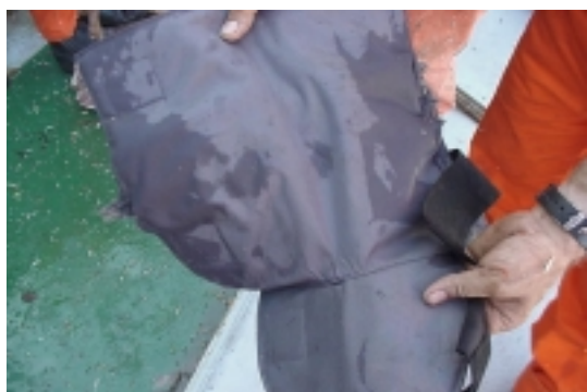
Photo 06 – The interior side of the Kevlar suit: We observe no destruction, only wet.
