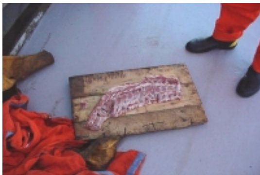
Photo 01 – Pig rib was fixed with nails to a wood table
